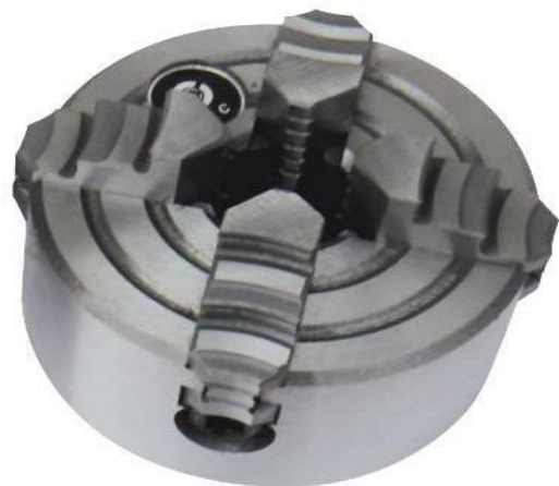
Figure 8-6: Four jaw independent chuck
