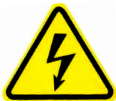
Figure 4 Warns user of hazardous voltage, and should be open up by trained personnel only.
