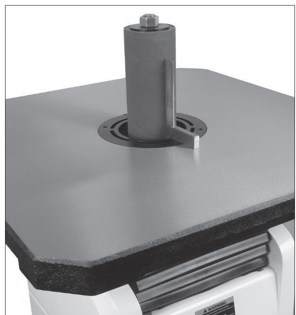
Figure 13: setting tilt stop
