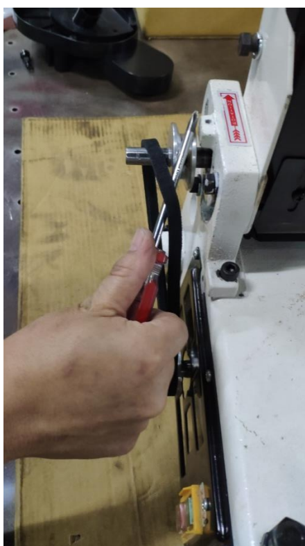
2. Use a screwdriver through the belt.
