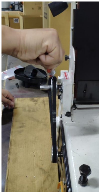
3. Then pull up the belt into the wheel groove.
