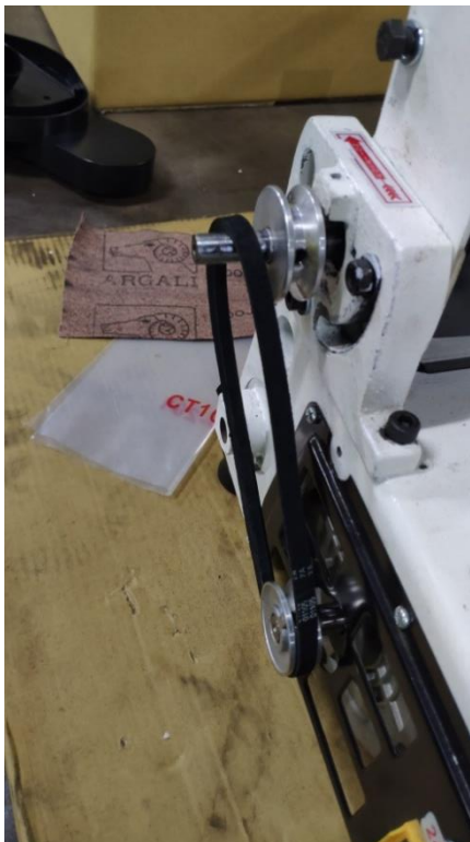
1. Put the belt on the drive wheel.
