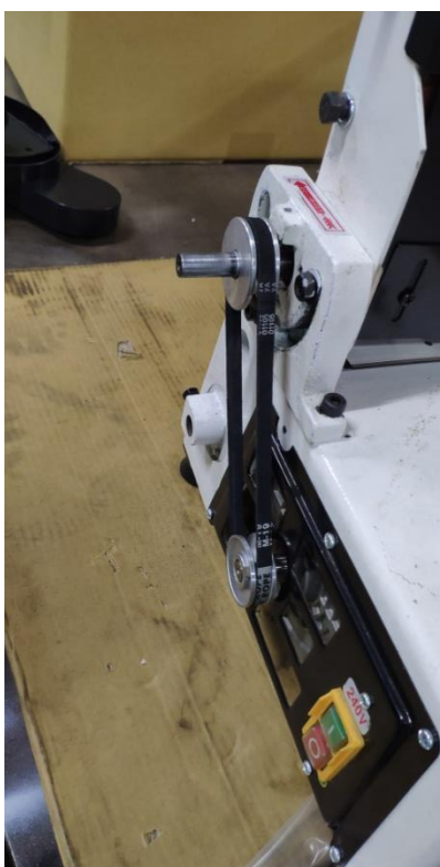
4. This action can make the belt to keep tight on the drive wheel. It has good friction when the belt contents with the wheel.
