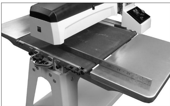
Figure 6-4: Aligned extension tables
