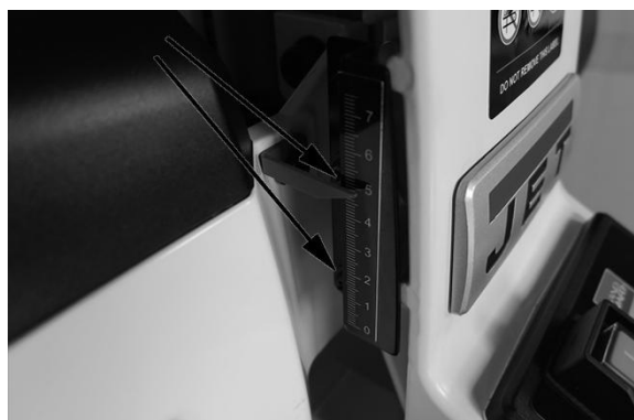
Figure 8-1: depth scale adjustment
