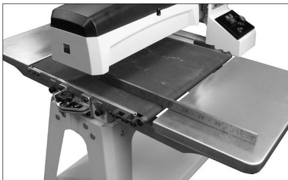
Figure 6-4: extension table alignment
