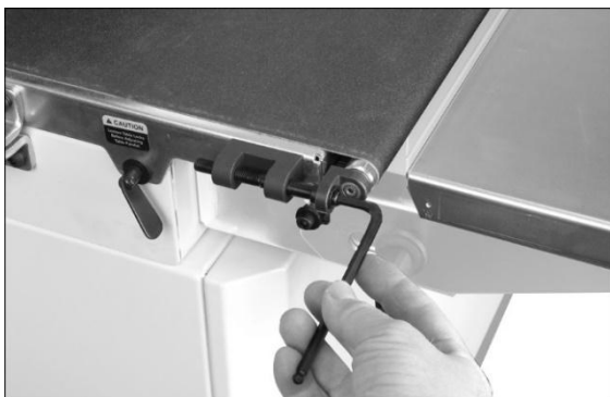
Figure 8-3: belt tension adjustment
