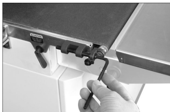
Figure 8-3: belt tension adjustment
