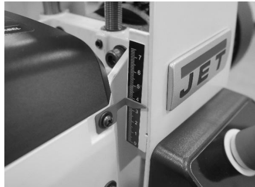
Figure 8-1: depth scale adjustment
